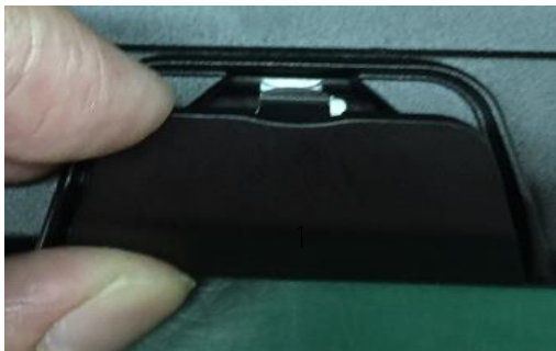
1. Remove barcode scanner cover.
