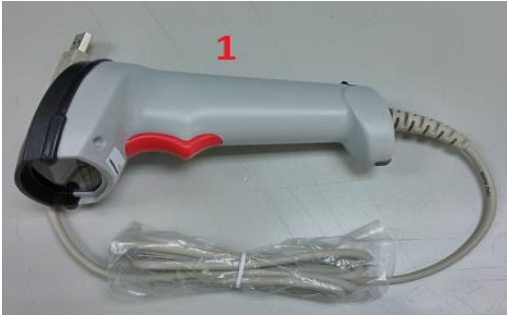
1. Plug the barcode scanner into a USB port.
