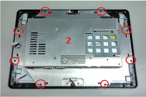
2. Dis-fasten chassis 8 screws.
