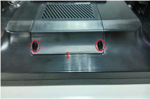
1. Dis-fasten 2 screws and remove base cover.
